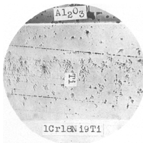
Figure 3 Micrograph of a cross-section of the alumina-1Cr18Ni9Ti joint with titanium filler ( \times 250 ); bonding temperature 875 °C; tensile strength 32.0 MPa.
