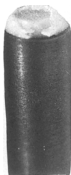
Figure 5 Bonded alumina-1Cr18Ni9Ti fractograph.
